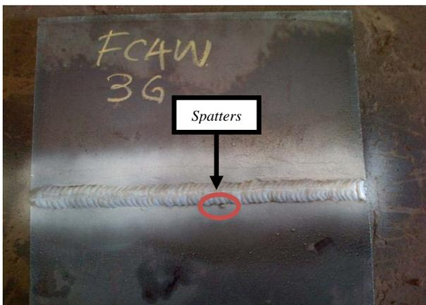
Gambar 5. Hasil Visual Test hasil lasan FCAW
