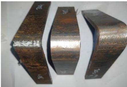
Gambar 14. Foto Makro *Bending HI-300 J/mm*
