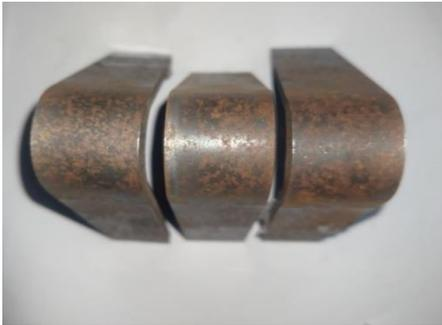
Gambar 12. Foto Makro *Bending Raw Material*
