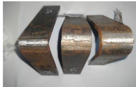
Gambar 15. Foto Makro *Bending HI-350 J/mm*
