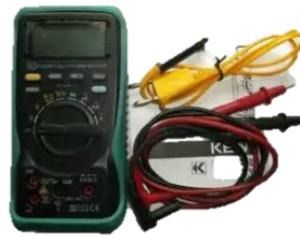
**Gambar 4.** Multi Tester Digital - Kyoritsu 1011
